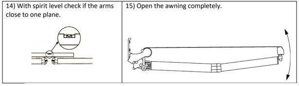
16) To change awning tilt angle loosen the M10x70 screw with Allen key. With the use of a flat wrench loosen (to increase tilt angle) or tighten (to decrease tilt angle) the regulation screws in arms brackets. Then tighten the M10x70 screw.
